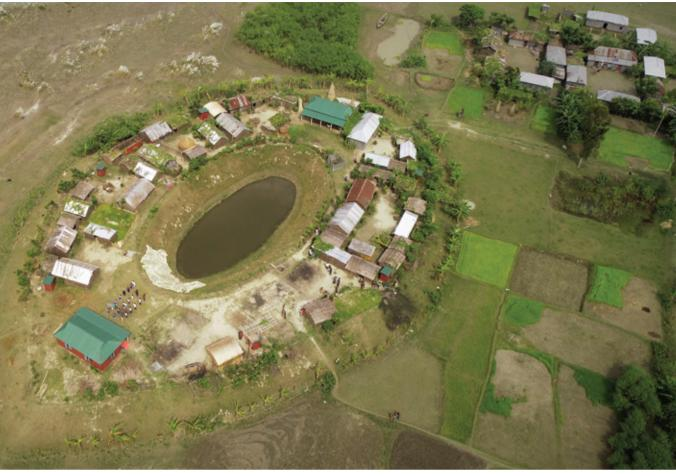
Plinths are cluster villages raised above flood levels, and designed to reduce loss of life and property during flooding.
